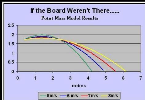
like darts a good approximation to the trajectory can be often gained assuming the projectile always points along its line of flight. This results in a "Point Mass" model (as on the left) where the only aerodynamic force considered is drag. Simpler still is an "In Vacuo" (ie no air and hence no aerodynamics) model where even drag is ignored and gravity is the only force considered. This gives rise to the solution of a parabola.
